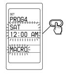
8 Set the hour by pressing the  $\bullet$  or  $\bullet$  (page 10). Then press the Joystick toward + so that the minute flashes. (You can switch the mode between the hour setting and the minute setting by pressing the Joystick toward  $\blacklozenge$  or  $\blacklozenge$ .) Set the minute by pressing the Joystick toward 🛧 or 🔸 (page 10). Then press down the Joystick. The time of the timer setting is decided.
